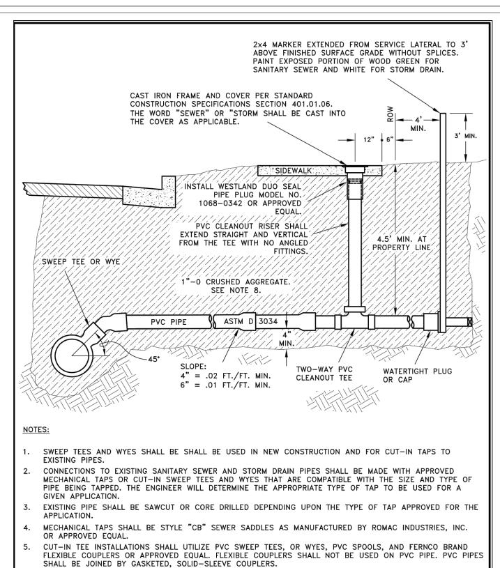
CLEANOUT FRAME AND COVER ASSEMBLIES SHALL BE INSTALLED IN CONCRETE SIDEWALKS. FRAME AND COVER
